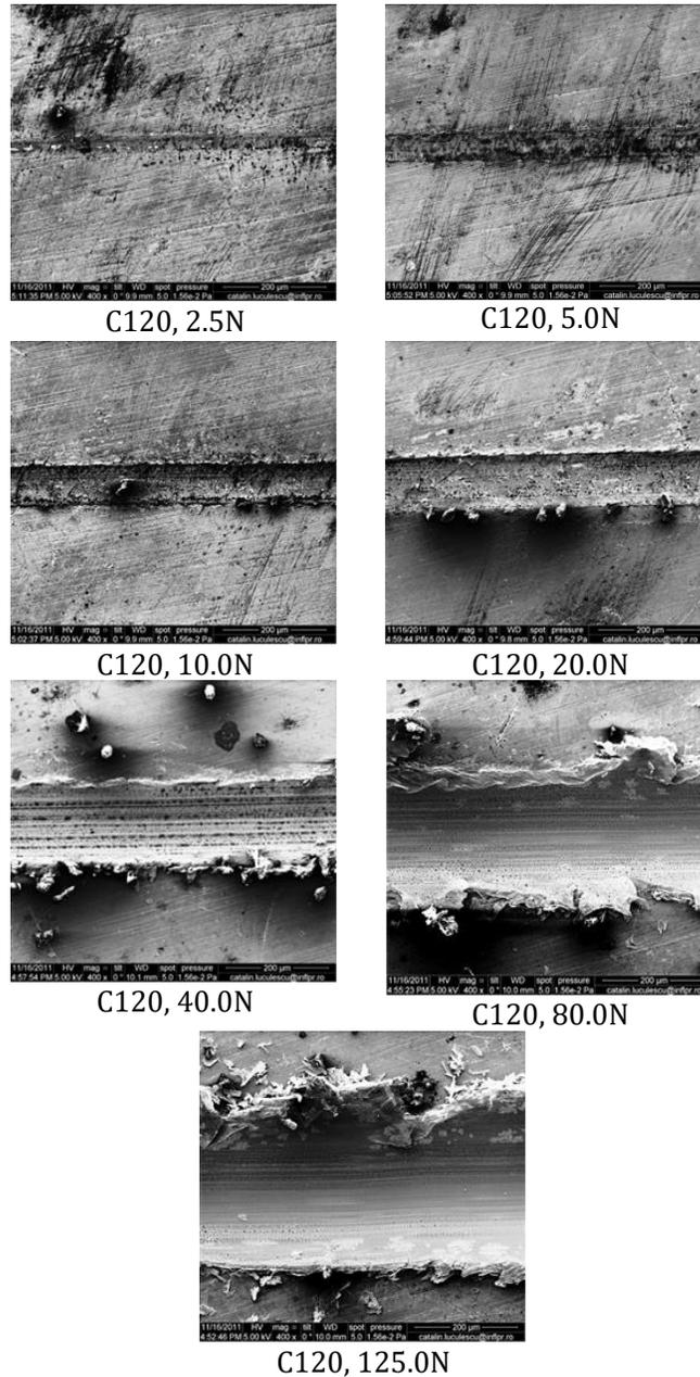
Figure 3: SEM microphotographs of the scratching scars on the surfaces of C120 steel samples (59 HRC) made at 10.0 N, 20.0 N, 40.0 N, 80.0 N, and 125.0 N loads, with the indenter having a radius of 2.5 mm.
