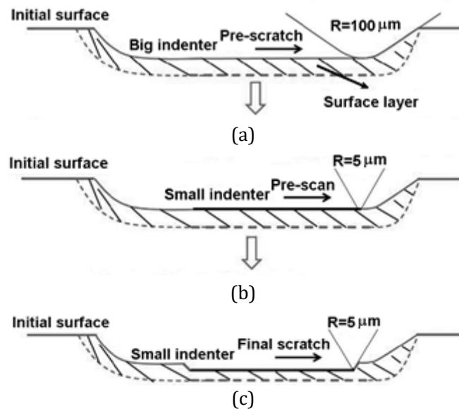
Figure 1: Configuration of multi-pass dual-indenter scratch test. Adapted after Xu, 2016.
