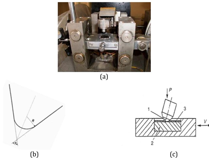
Figure 2: Scratching tester with a diamond spherical segment. (a) General view; (b) Indenter tilt; (c) Functional scheme: 1 – natural diamond spherical segment; 2 – sample of tested material; 3 – lubricant (bovine serum). The plate has an oscillatory movement.
