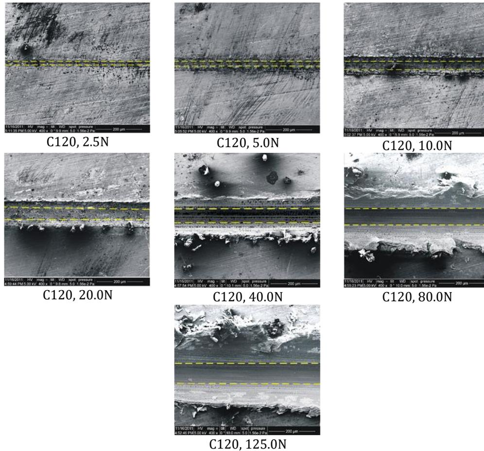
Figure 6: SEM microphotographs of the scratching scars on the surfaces of C120 steel samples (59 HRC) made at 10.0 N, 20.0 N, 40.0 N, 80.0 N, and 125.0 N loads, with the indenter having a radius of 1 mm (dual indentation), after 10 passes (multi-pass), i.e. multi-pass dual-indenter.
