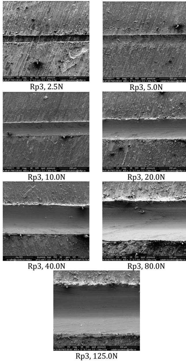
Figure 4: SEM microphotographs of the scratching scars on the surfaces of Rp3 steel samples (62 HRC) made at 10.0 N, 20.0 N, 40.0 N, 80.0 N, and 125.0 N loads, with the indenter having a radius of 2.5 mm.
