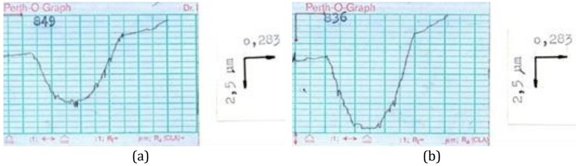
Figure 5: Recordings of the cross-sectional profile of the scratching scar made by the large indenter on the (a) Rp3 and (b) C120 steels, at 5.0 N.
