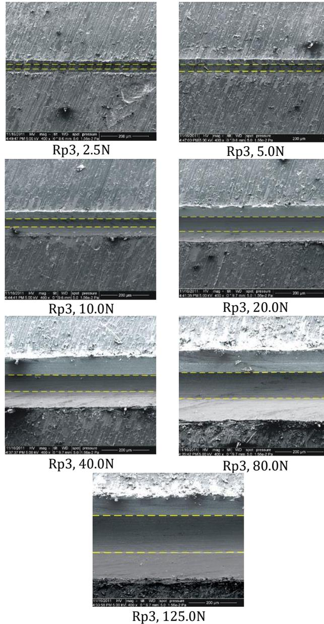
Figure 7: SEM microphotographs of the scratching scars on the surfaces of Rp3 steel samples (62 HRC) made at 10.0 N, 20.0 N, 40.0 N, 80.0 N, and 125.0 N loads, with the indenter having a radius of 1 mm (dual indentation), after 10 passes (multi-pass), i.e. multi-pass dual-indenter.
