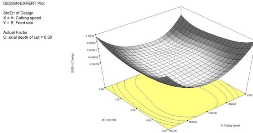
Figure 3: 3D surface plot of surface roughness ( $\mu\text{m}$ ) with feed rate and cutting speed.
