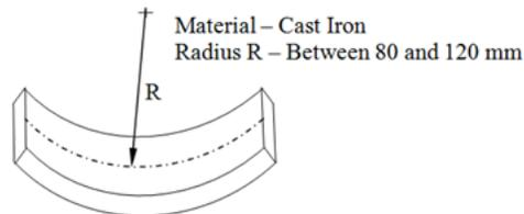
Figure 4: Liner specimen.
