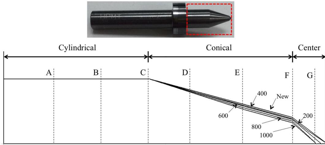
Figure 4: Tool profile measured at seven locations.
