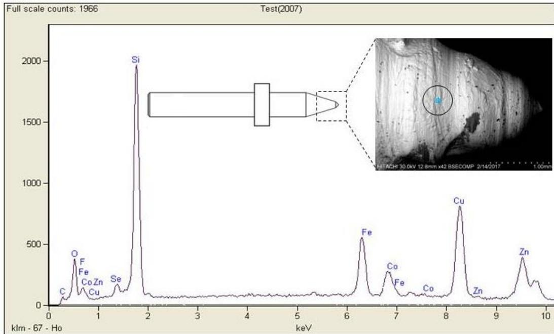
Figure 9: SEM image and EDS analysis.
