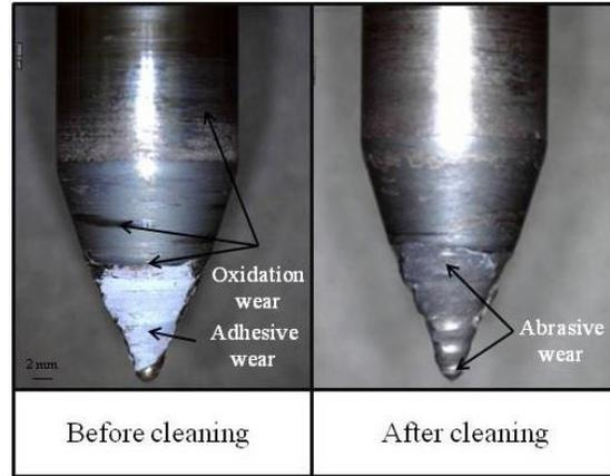
Figure 10: Oxidation wear.
