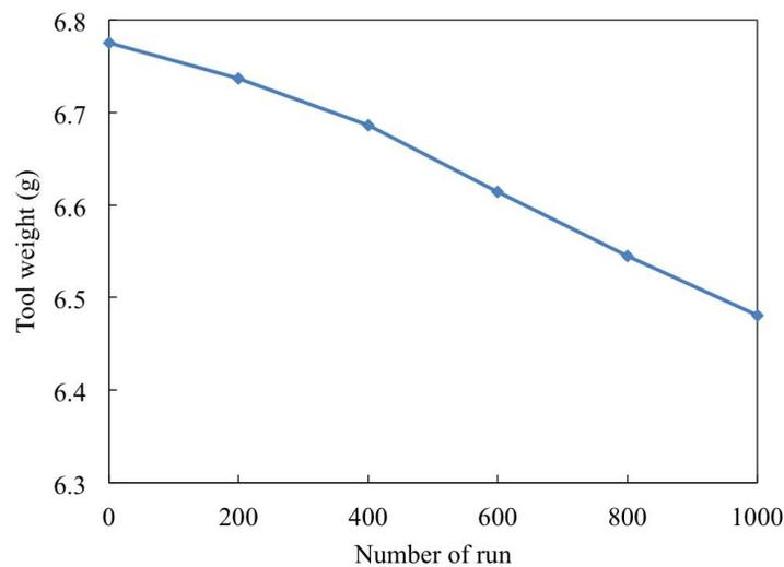
Figure 5: The weight lost until drilling 1000 holes.
