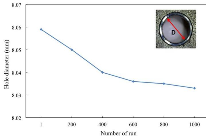
Figure 6: Hole diameter at the number of run.
