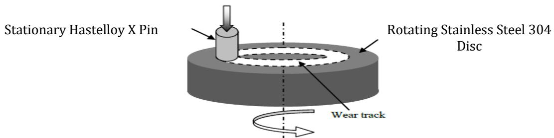
Figure 1: Schematic diagram of pin and disc. Adapted Mat Tahir et al., 2014.
