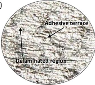
Adhesive terrace<br/>Delaminated region</p> <p>4 mm</p> | <p>(d)
