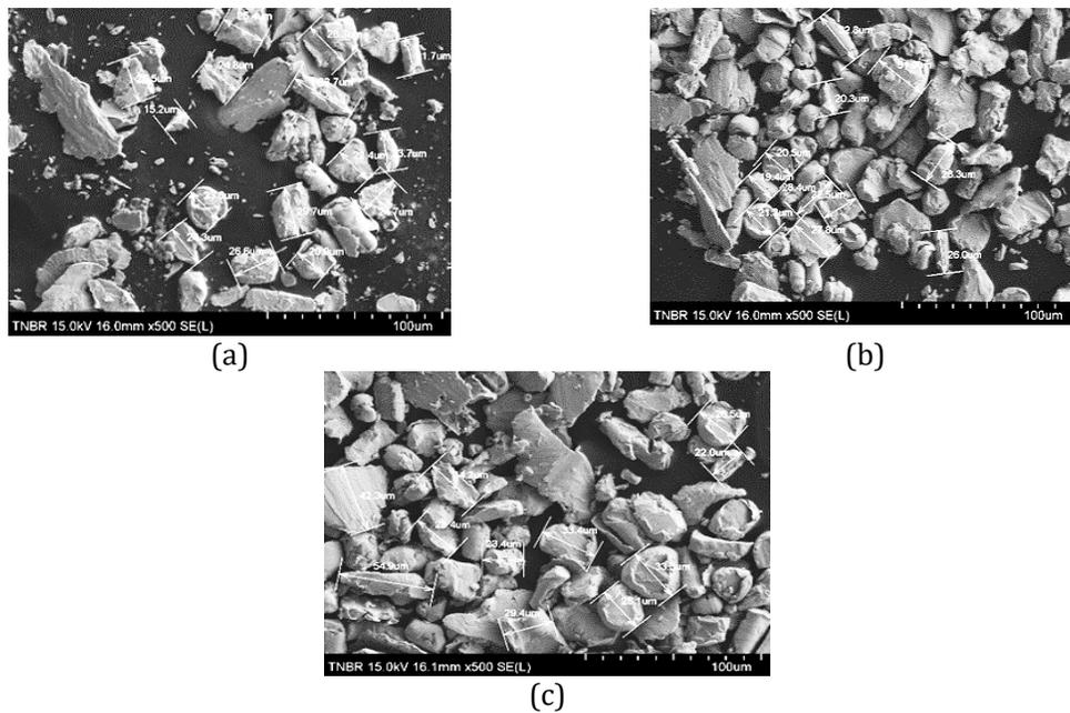
Figure 5: Wear debris analysis of SS 304-Hastelloy X at 25 °C for (a) 1 hour, (b) 3 hours and (c) 5 hours.
