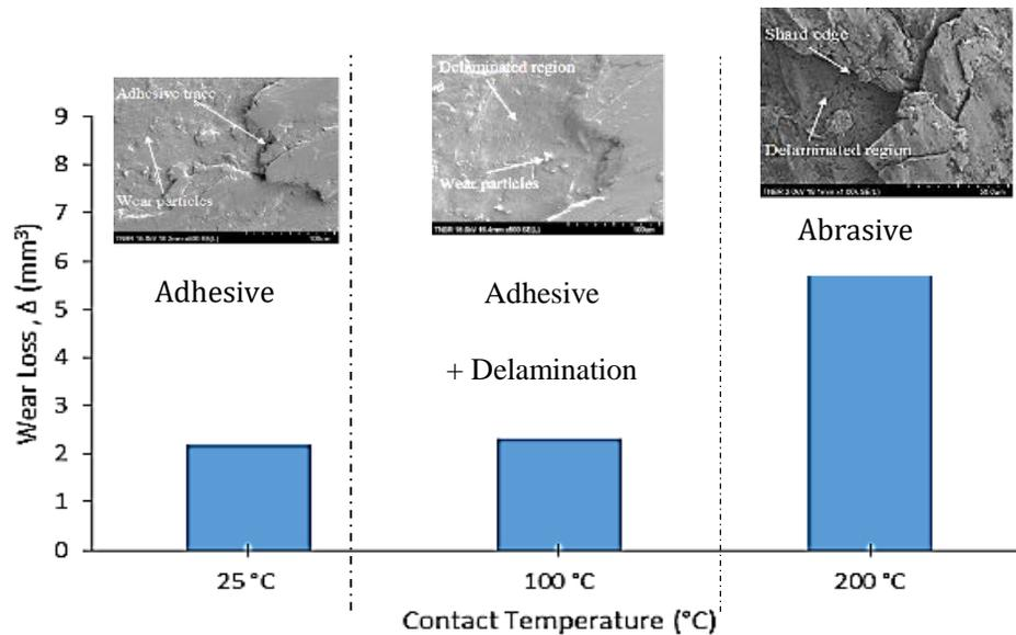
Figure 7: Wear transition of SS 304-Hastelloy X tribo-pair (pin side).
