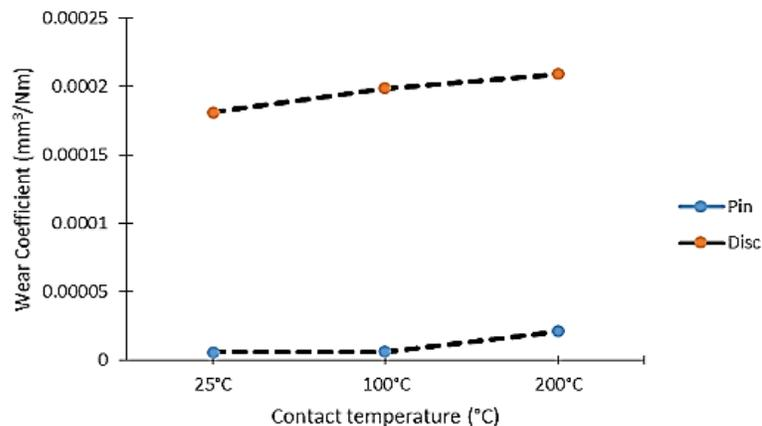
Figure 3: Wear coefficient against contact temperature of SS 304-Hastelloy X tribo-pair at 5 hours.
