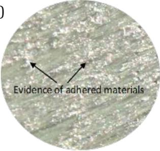
Evidence of adhered materials</p> <p>4 mm</p>            | <p>(b)
