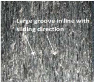
Large groove in line with sliding direction</p> <p>6 mm</p>              |
