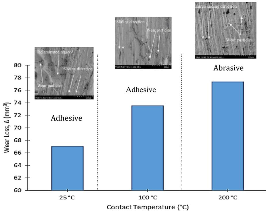
Figure 8: Wear transition of SS 304-Hastelloy X tribo-pair (disc side).
