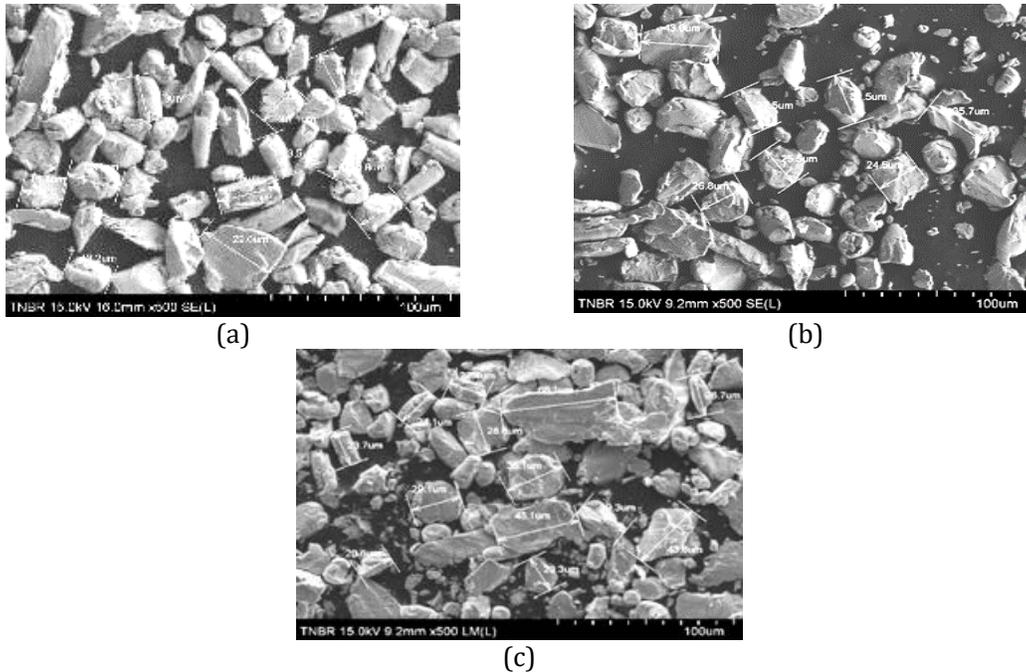
Figure 7: Wear debris analysis of SS 304-Hastelloy X at 200 °C for (a) 1 hour, (b) 3 hours and (c) 5 hours.
