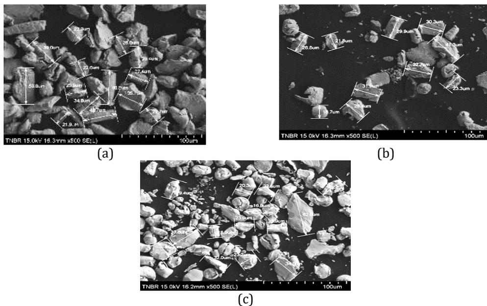
Figure 6: Wear debris analysis of SS 304-Hastelloy X at 100 °C for (a) 1 hour, (b) 3 hours and (c) 5 hours.
