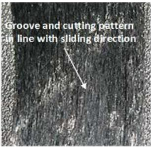
Groove and cutting pattern in line with sliding direction</p> <p>6 mm</p> |
