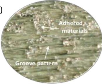
Adhered materials<br/>Groove pattern</p> <p>4 mm</p>   | <p>(f)
