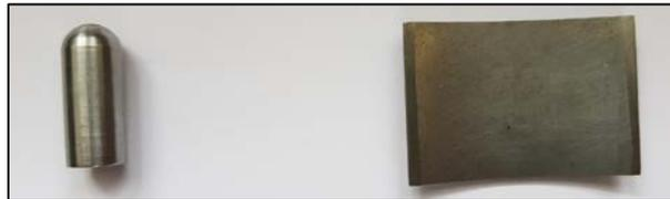
Figure 1: Pin and cylinder sleeve samples after cutting and machining.
