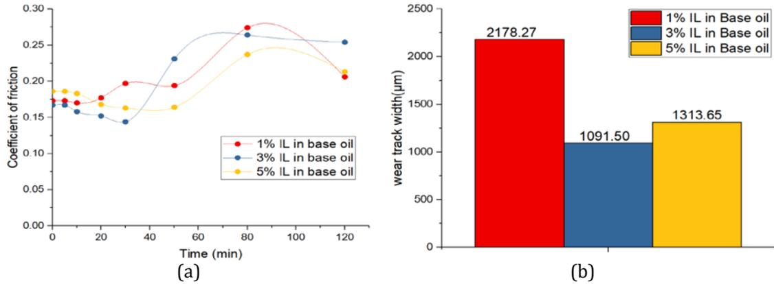
Figure 4: (a) Comparison of COF of samples tested with 1%, 3% and 5% IL in base oil, (b) Comparison of wear track width of samples tested with 1%, 3% and 5% IL in base oil
