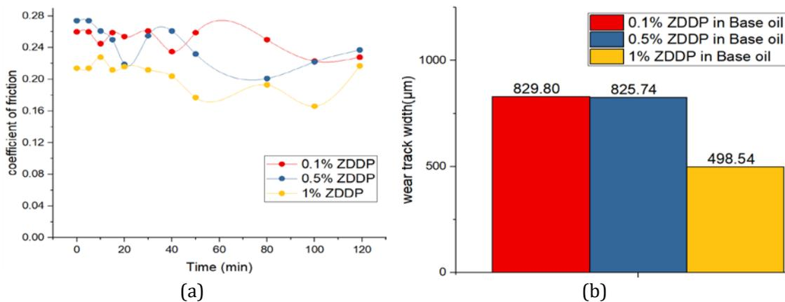
Figure 5: (a) Comparison of COF of samples tested with 0.1%, 0.5% and 1% ZDDP in base oil, (b) Comparison of wear track width of samples tested with 0.1%, 0.5% and 1% ZDDP in base oil.
