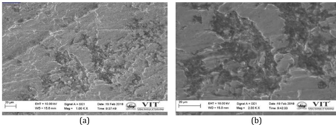
Figure 8: SEM of the wear scar on the cylinder sleeve surface with 1% IL (a) 1000X (b) 2000X.
