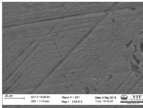
Figure 11: SEM image of the unworn surface of sleeve specimen at 2000X.
