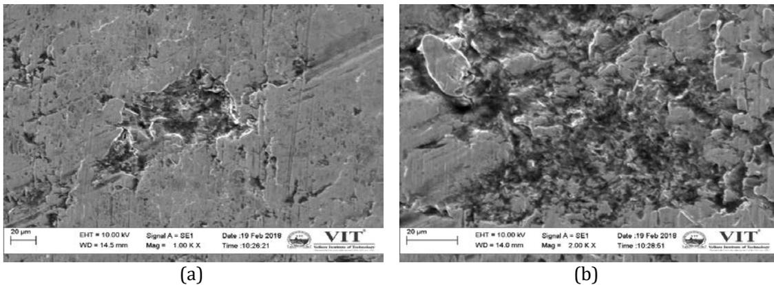
Figure 10: SEM of the wear scar on the cylinder sleeve surface with 5% IL (a) 1000X; (b) 2000X.
