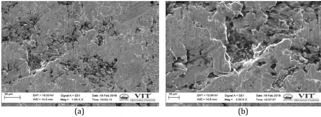
Figure 9: SEM of the wear scar on the cylinder sleeve surface with 3% IL (a) 1000X (b) 2000X.
