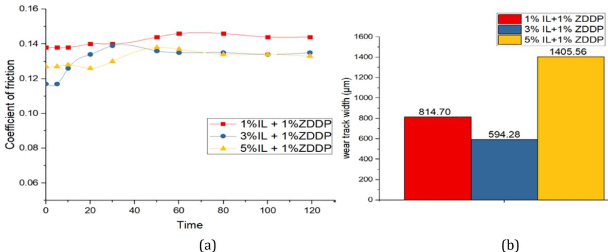
Figure 6: (a) Comparison of COF values of specimens tested with blends of IL and ZDDP in base oil (b) Comparison of wear track width of specimens tested with blends of IL and ZDDP in base oil
