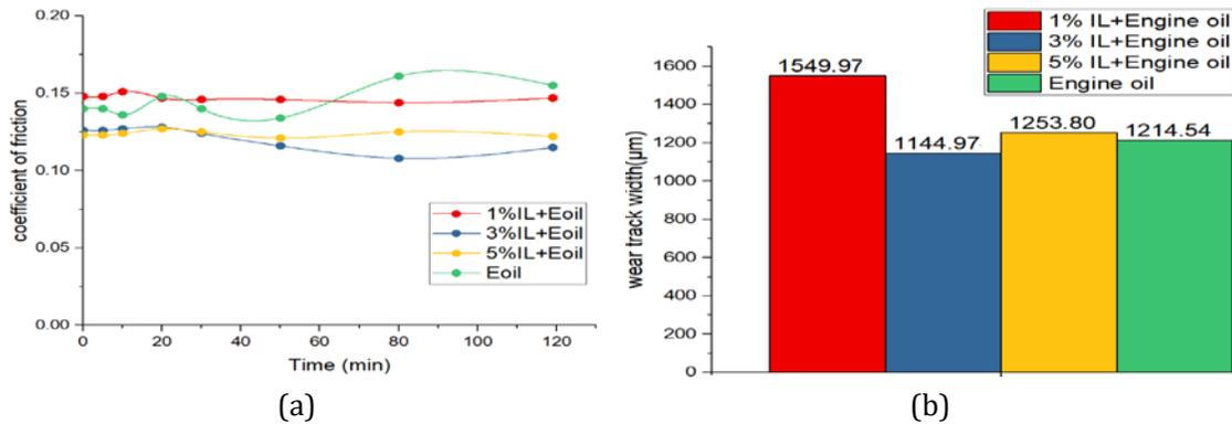
Figure 7: (a). Comparison of COF values of specimens tested with blends of IL and engine oil, (b) Comparison of wear track widths of specimens tested with blends of IL and engine oil
