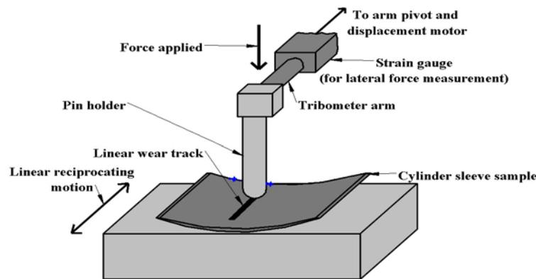
Figure 3: Sample setup on the wear testing machine.
