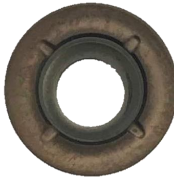
Figure 2: RDET 10T3 M0EN-G tool insert with 10 mm diameter.
