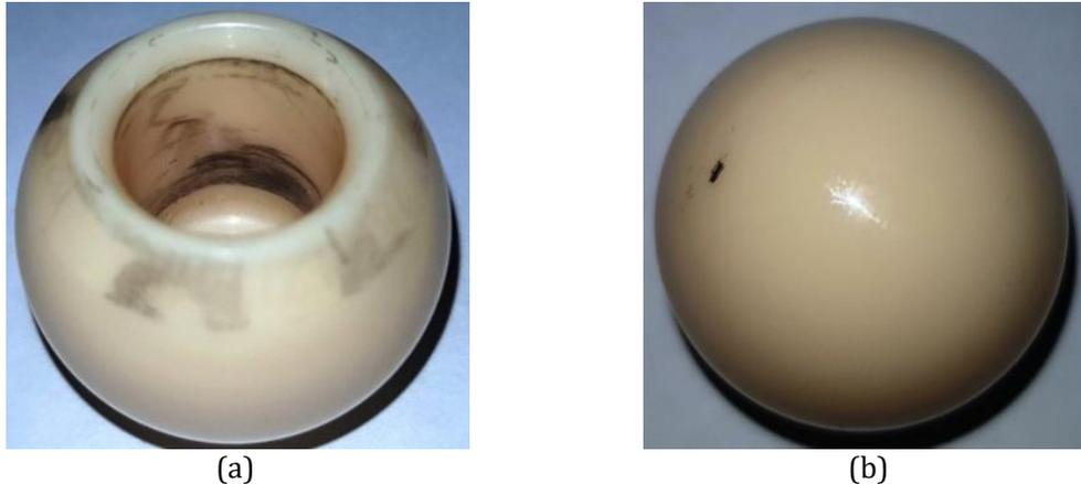
Figure 7: (a) An internal taper of the femoral head tested at impact on the stem, showing grey marks of micro-movement and fretting wear, prior to cleaning, and (b) a metallic wear particle embedded in the outer surface of the ceramic head.
