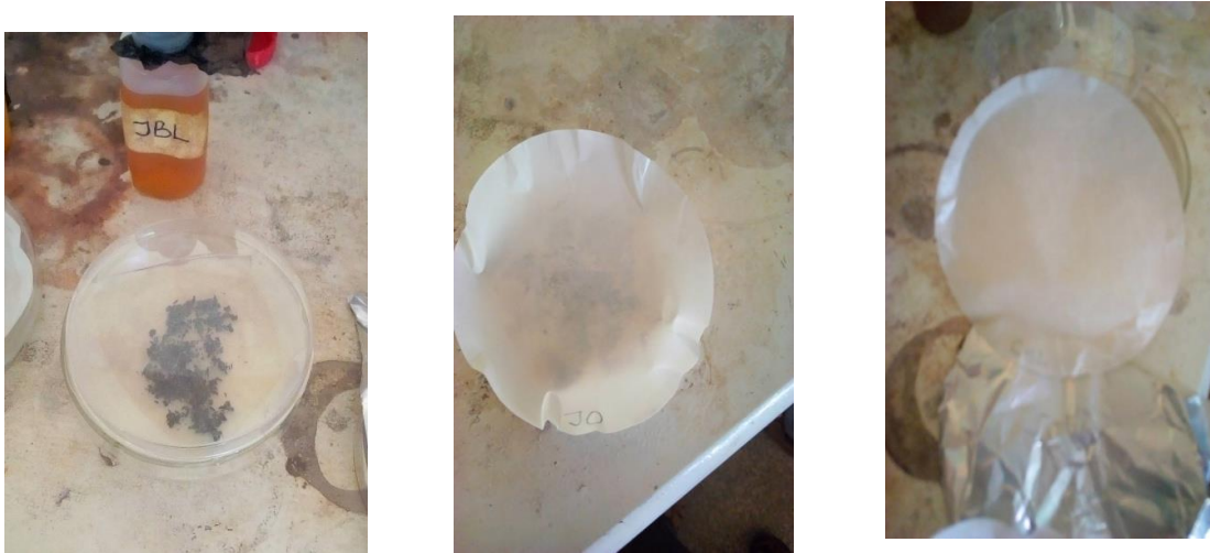
(a) Test with cast iron particles (b) after 2Hrs, Jatropha oil (c) after 2Hrs, SAE20W50 Figure 4: Corrosion inhibition tests of jatropha oil and SAE 20W50.
