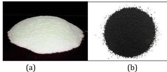
Figure 1: (a) UHMWPE powder and (b) carbon black powder.
