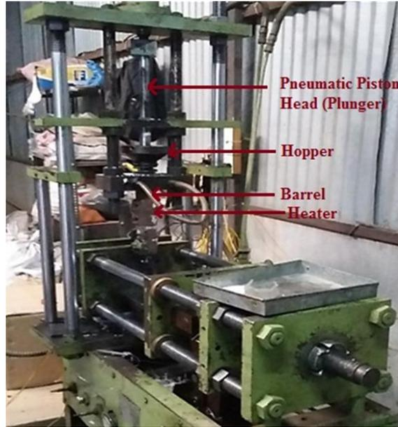
Figure 3: Injection moulding machine.
