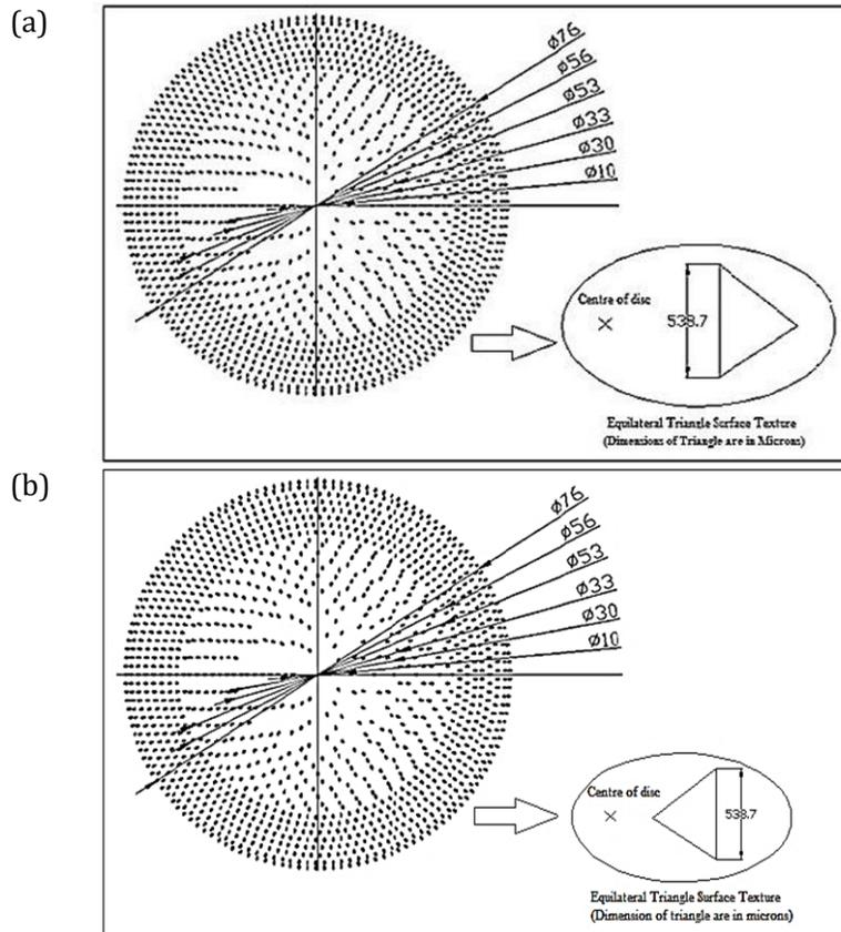
Figure 6: Orientation of equilateral triangle surface texture on the disc with (a) base of triangle and (b) apex of triangle towards center of the disc.
