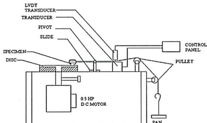
Figure 7: Pin on disc wear test rig.
