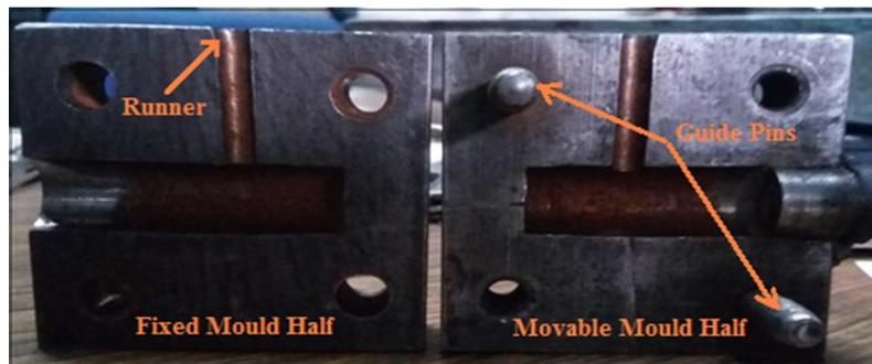
Figure 2: Mould for manufacturing UHMWPE composite pins.
