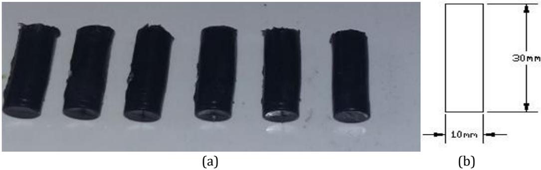
Figure 4: (a) UHMWPE composites pins (b) schematic diagram of pin with dimension.
