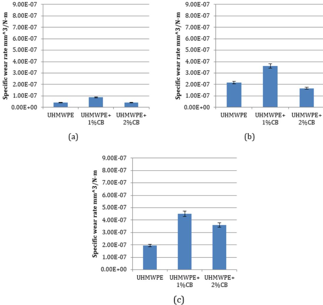
Figure 10: Specific wear rates with the orientation of surface texture equilateral triangle base towards the center of disc for (a) 0% dimple density (b) 10% dimple density (c) 20% dimple density.
