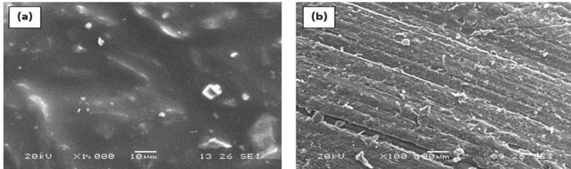
Figure 12: SEM micrographs of worn surfaces of UHMWPE + 2% CB, Load=181.42 N, Density=20% & Sliding Velocity=0.09 m/s (a) before wear test (b) after wear test.
