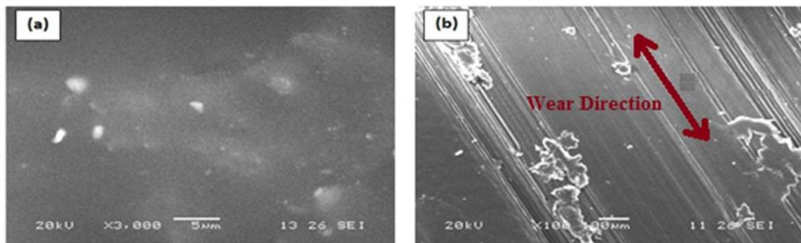
Figure 11: SEM micrographs of worn surfaces of UHMWPE + 2% CB, Load=171.62N, Density=10% and Sliding Velocity=0.12m/s (a) before wear test (b) after wear test.
