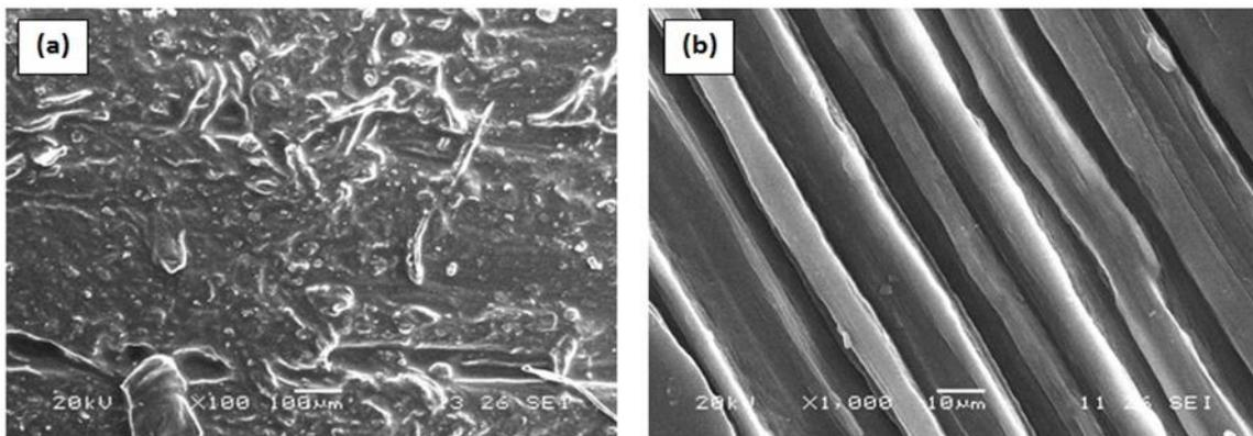
Figure 13: SEM micrographs of worn surfaces of UHMWPE, Load=156.91N, Density=10% & Sliding Velocity=0.09 m/s (a) before wear test (b) after wear test
