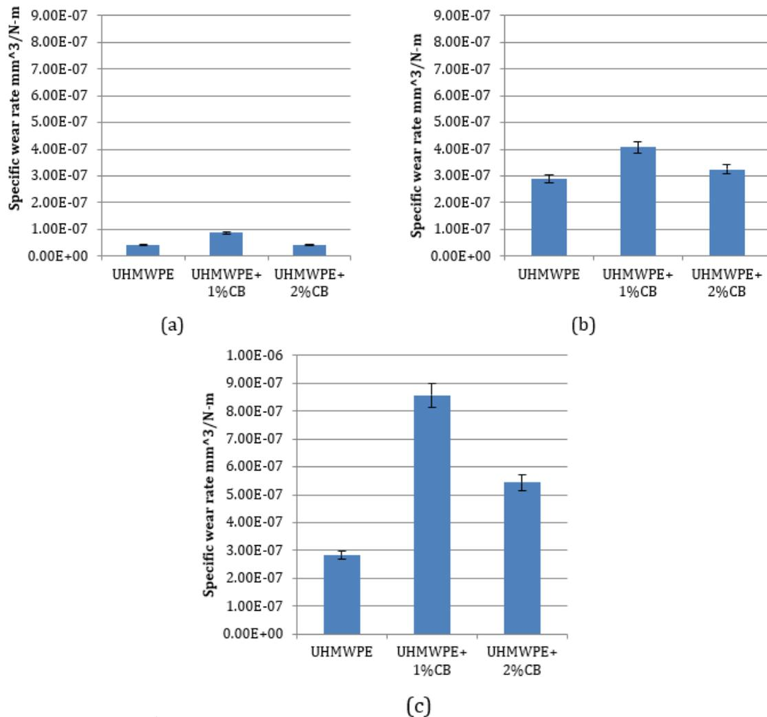
Figure 9: Specific wear rates with the orientation of surface texture equilateral triangle apex towards the center of disc for (a) 0% dimple density (b) 10% dimple density (c) 20% dimple density.
