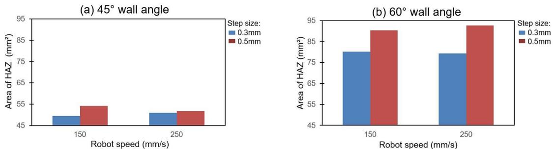
Figure 4: Effects of processing parameters on HAZ for producing truncated cone profile.
