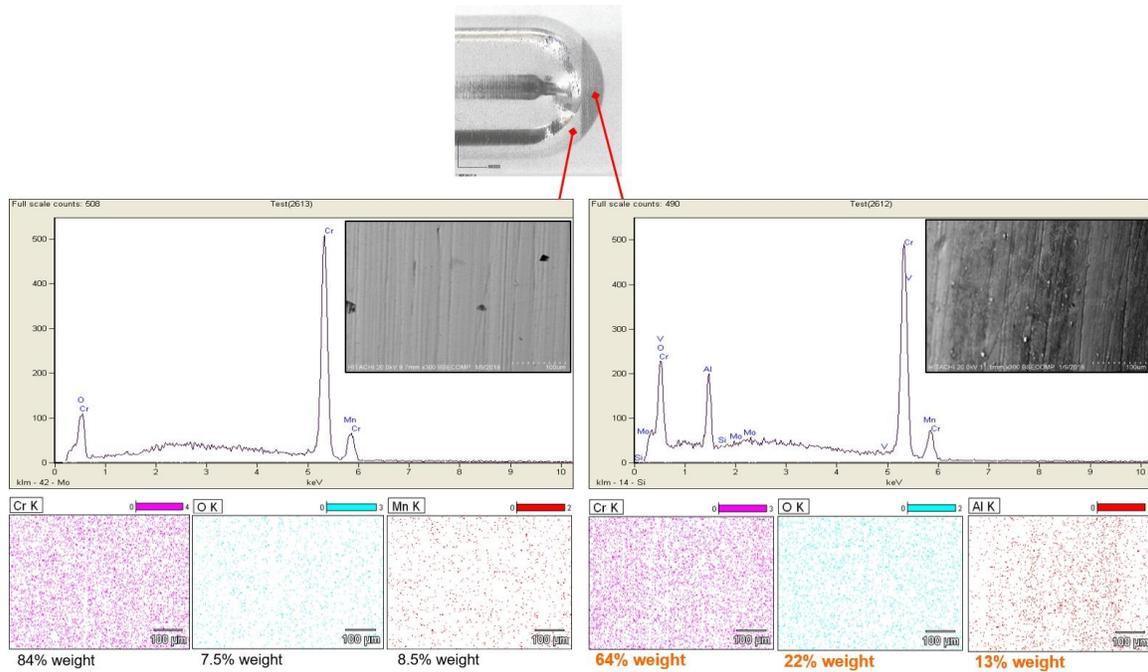
Figure 5: The SEM images and EDS analysis with three main elements detected at HAZ and non-HAZ of forming tools.
