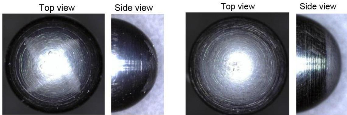
Figure 3: The HAZ pattern generated on the forming tool after the robot based ISF process.
