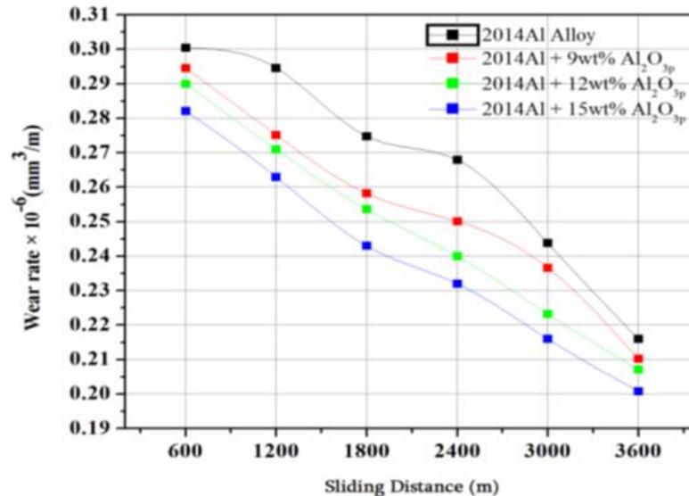
Figure 6: Effect of sliding distance on the Al2014 matrix wear rate before and after addition of Al<sub>2</sub>O<sub>3</sub> particulates.
