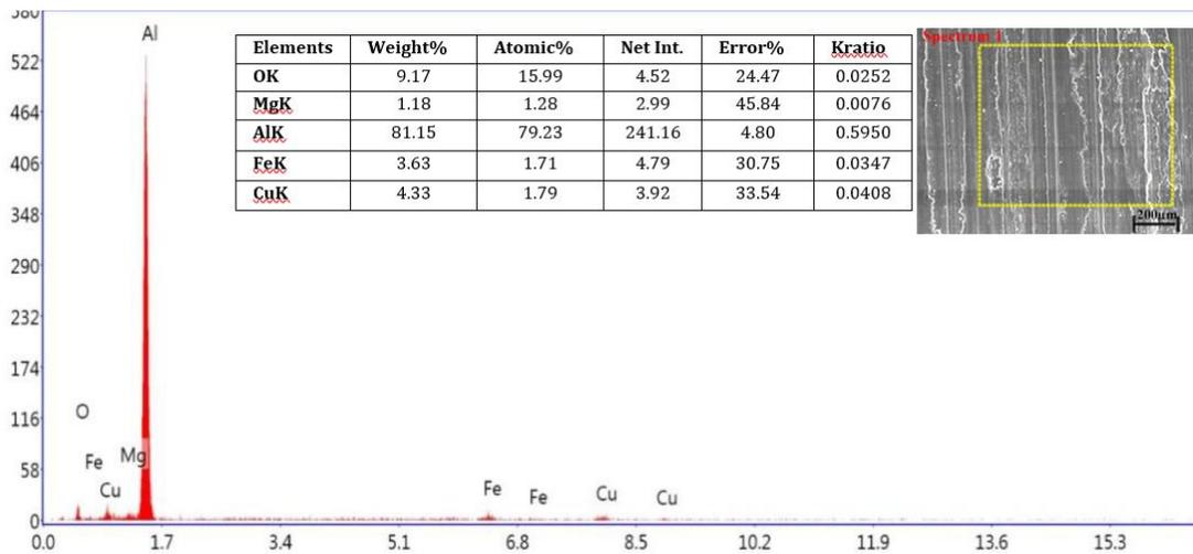
Figure 9: EDS Analysis of worn surface of Al2014-15wt. % Al<sub>2</sub>O<sub>3p</sub>.
