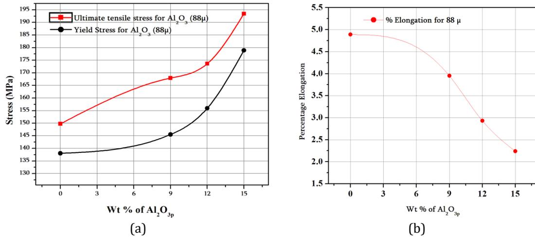
Figure 4: (a) Tensile test and (b) % elongation outcomes of Al2014-alloy before and after addition of different wt% of Al<sub>2</sub>O<sub>3p</sub> (88µ).
