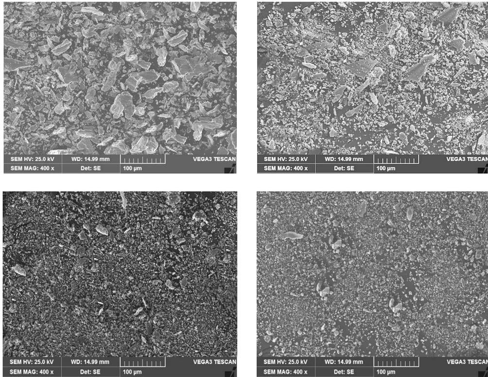
Figure 10: Wear debris morphology of (a) as cast Al2014 alloy, b Al2014 alloy with 9 wt. % Al<sub>2</sub>O<sub>3p</sub>, (c) Al2014 alloy with 12 wt. % Al<sub>2</sub>O<sub>3p</sub> and (d) Al2014 alloy with 15 wt. % Al<sub>2</sub>O<sub>3p</sub>.
