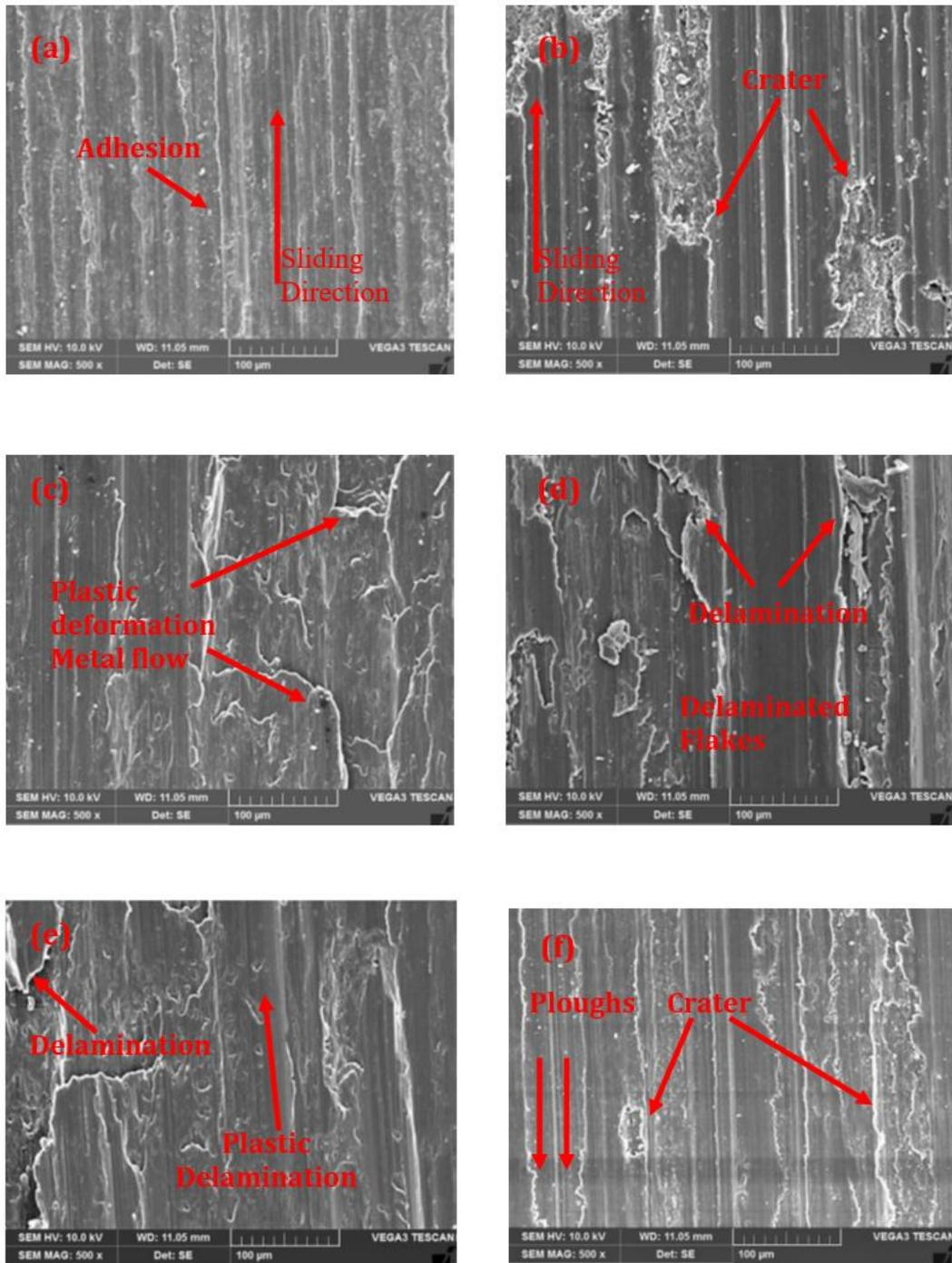
Figure 8 SEM Photographs of wear tracks of Al2014-Al<sub>2</sub>O<sub>3p</sub> composites showing different wear mechanisms.
