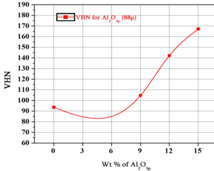
Figure 3: Discrepancies in Al2014 hardness prior and after addition of specific  $Al_2O_{3p}$  weight percent (88 $\mu$ ).
