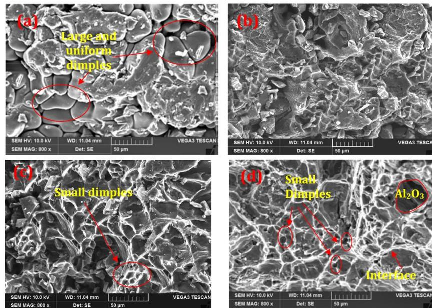
Figure 5: Fractured surfaces of samples of (a) Al2014 matrix alloy, (b) Al2014-9 wt. % of Al<sub>2</sub>O<sub>3</sub>, (c) Al2014-12wt. % of Al<sub>2</sub>O<sub>3</sub> and (d) Al2014-15 wt.% of Al<sub>2</sub>O<sub>3</sub> particulate composites.
