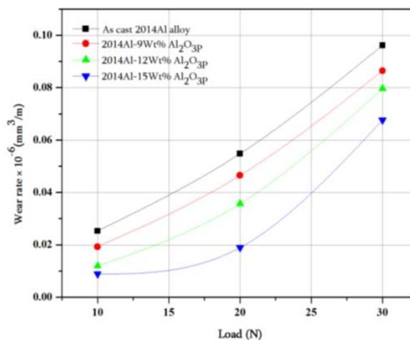
Figure 7: Comparison between wear rates of as cast Al2014 matrix and Al2014 composites reinforced with 9, 12 and 15wt. % of Al<sub>2</sub>O<sub>3</sub> particulates.
