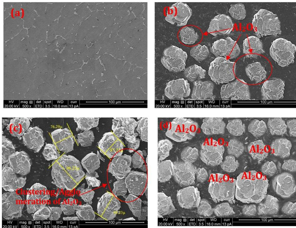
Figure 1: SEM images of (a) as cast Al2014 alloy, (b) Al2014 alloy with 9 wt. % Al<sub>2</sub>O<sub>3p</sub>, (c) Al2014 alloy with 12 wt. % Al<sub>2</sub>O<sub>3p</sub> and (d) Al2014 alloy with 15 wt. % Al<sub>2</sub>O<sub>3p</sub>.
