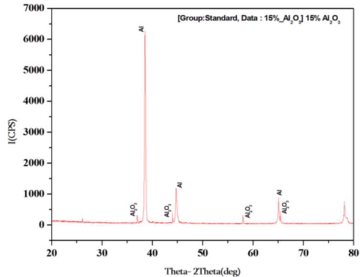
Figure 2: X-ray diffraction pattern of the Al2014 alloy with 15 wt. % Al<sub>2</sub>O<sub>3</sub>.
