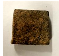
Figure 1: Camera ready photo of the silicizing process at 1000°C for 4 hours.
