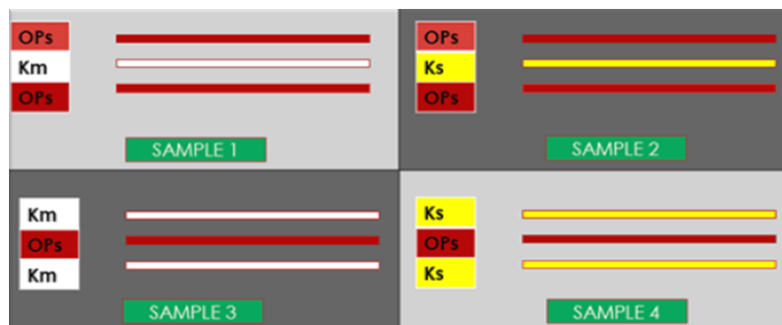
Figure 2: Various hybrid OPEFB/kenaf reinforced epoxy composites layering sequence.
