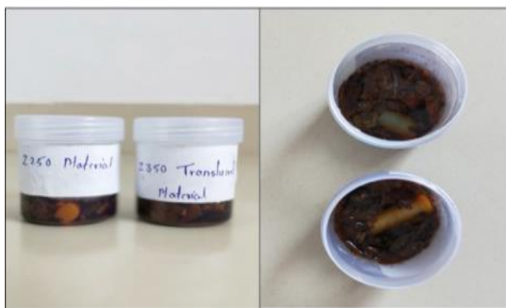
Figure 1: Specimens dipped in tobacco solution.
