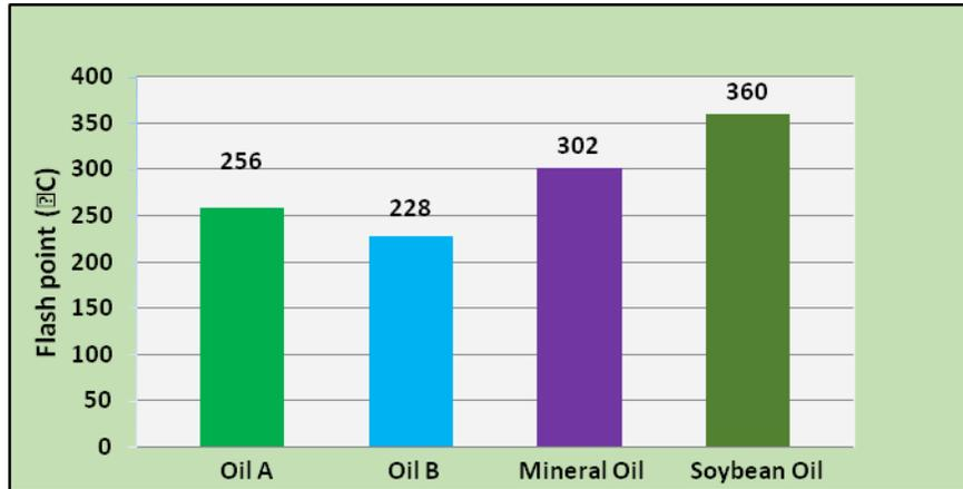
Figure 4: Flash point of selected blends (ASTM D92-12b)
