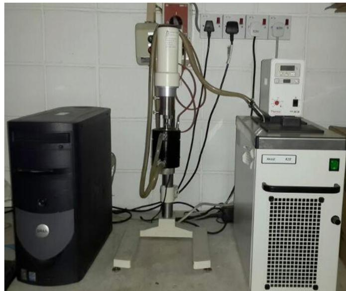
Figure 2: Controlled-stress rheometer
