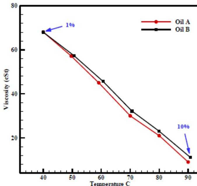
Figure 3: Temperature dependent viscosity of the formulated oil in comparison with ISO VG 68
