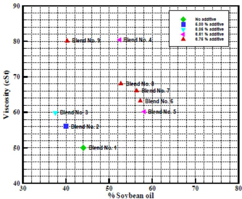
Figure 1: Viscosity of various blends at 40 °C (ASTM D445-15a)
