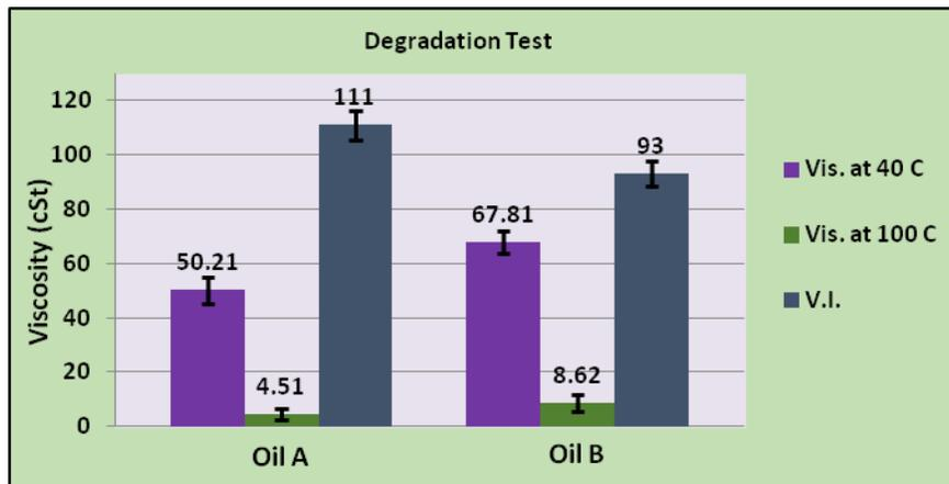
Figure 5: Changes of viscosity and viscosity index for lubricants A and B
