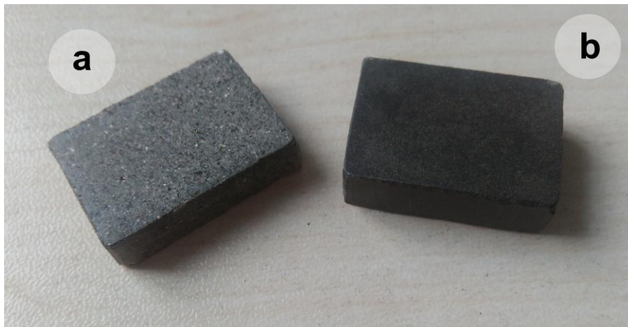
Figure 1: Specimen used in the experimental works (a) compact form (b) sintered form.
