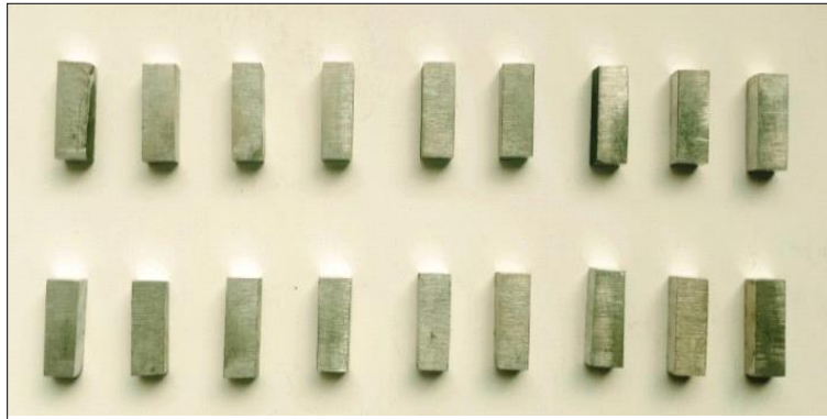
Figure 1: Pin-type samples used in the wear testing.
