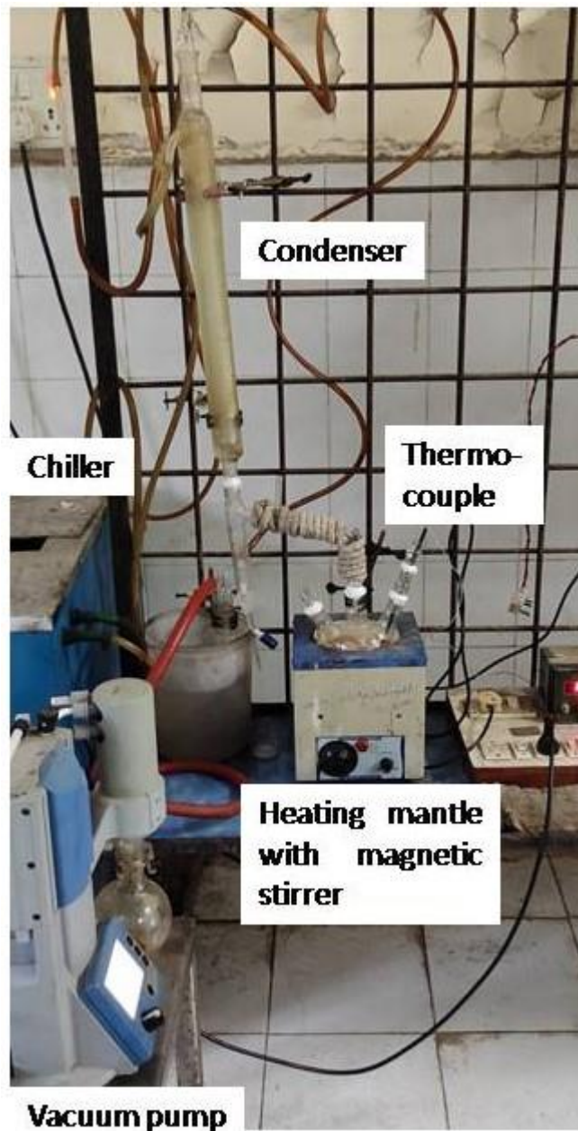
Figure 1: Experimental setup for TMP ester synthesis.
