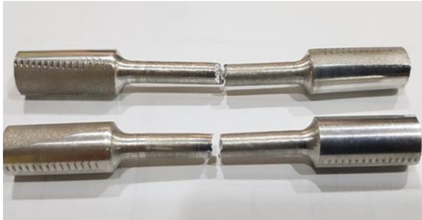
Figure 10: Fractured samples of the thixoformed Al-5Si-Cu-1.0Mg.
