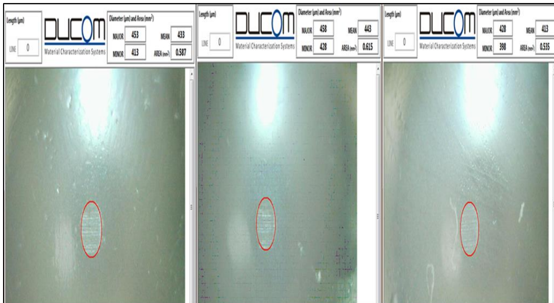
Figure 7: Wear Behaviour for gear EP Lubricant blended with composite additive.
