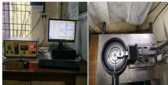
Figure 4: Pin on Disk wear testing setup.
