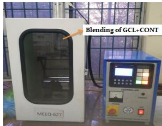
Figure 2: Prob Sonicator blending process.
