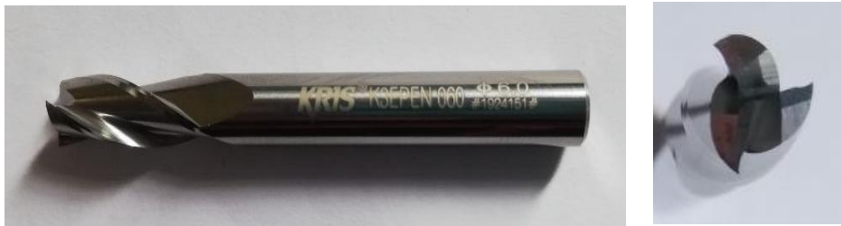
Figure 1: 6 mm tungsten carbide end mill tool supplied by Precisetech.
