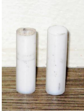
Figure 2: Specimen PTFE cylindrical pin.
