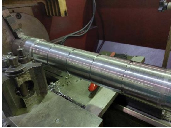
Figure 3: The segmented Inconel 718 clamped in the lathe machine (HARRISON M390).
