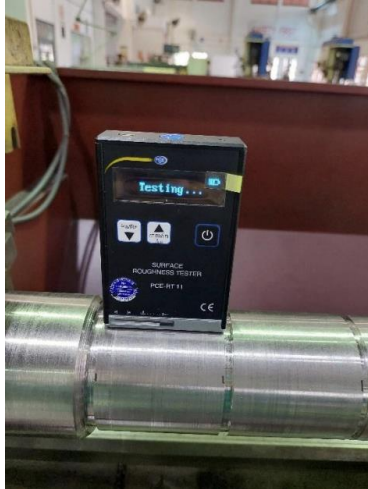
Figure 5: Measuring the surface roughness on the machined surface of Inconel 718.
