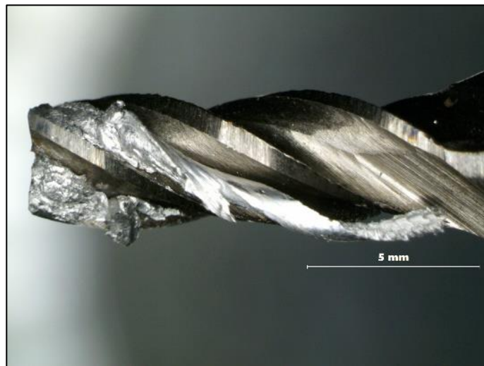
Figure 5: Welded chips and material adhesion under dry cutting.
