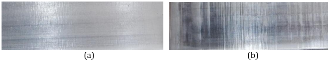
Figure 4: Surface of experimental results. (a) number 2, which was done on the spindle speed at 3000 rpm, with a feeding speed of 100 mm/min, the depth of cut of 0.5 mm, and MQL spraying to the feed direction, (b) number 12, which was done on the spindle at 3000 rpm, with a feeding speed of 150 mm/min, the depth of cut of 0.5 mm, and MQL spraying to the opposite direction of feeding.
