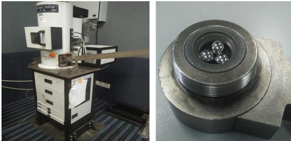
Figure 3: The four-ball tribo-tester and the oil rig.
