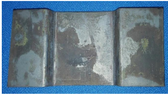
Figure 4: The 22MnB5 boron steel after the hot press forming processes.
