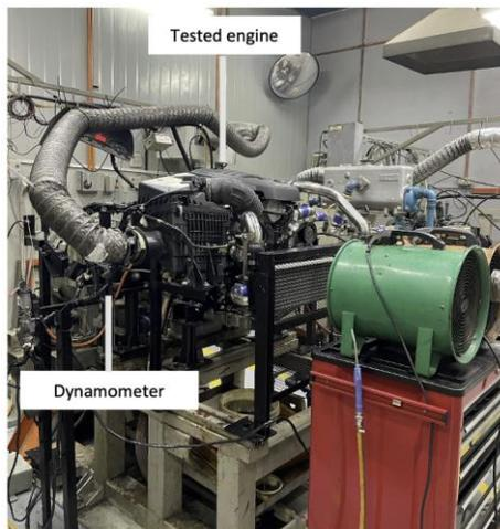
Figure 2: Real setup of the engine-dynamometer endurance test bed.
