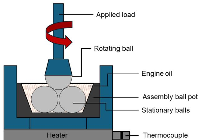
Figure 3: Schematic diagram of fourball test.
