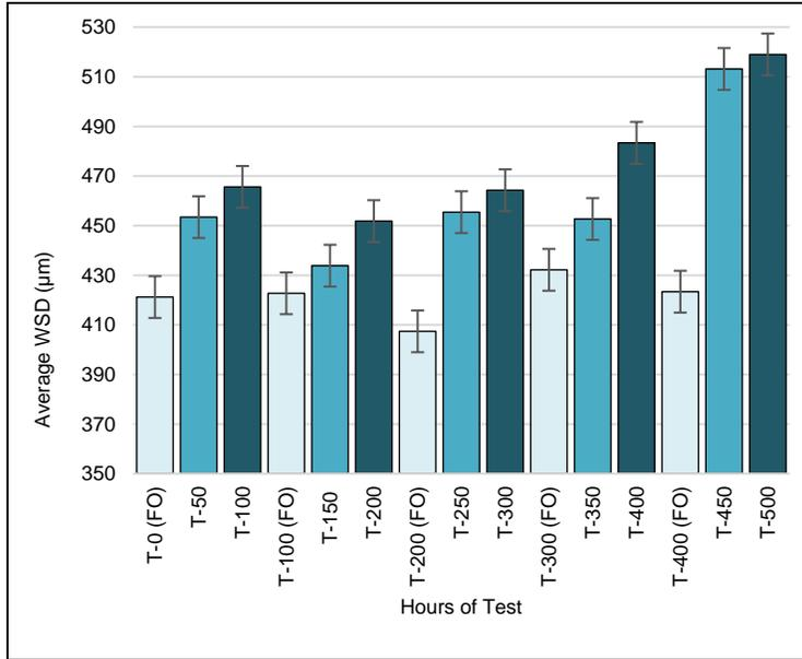
Figure 7: Average WSD of the tested ball for engine oil samples over the 500-hour endurance test.
