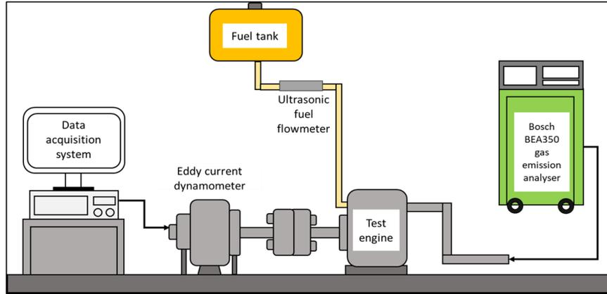
Figure 1: Schematic diagram of engine-dynamometer endurance test bed.
