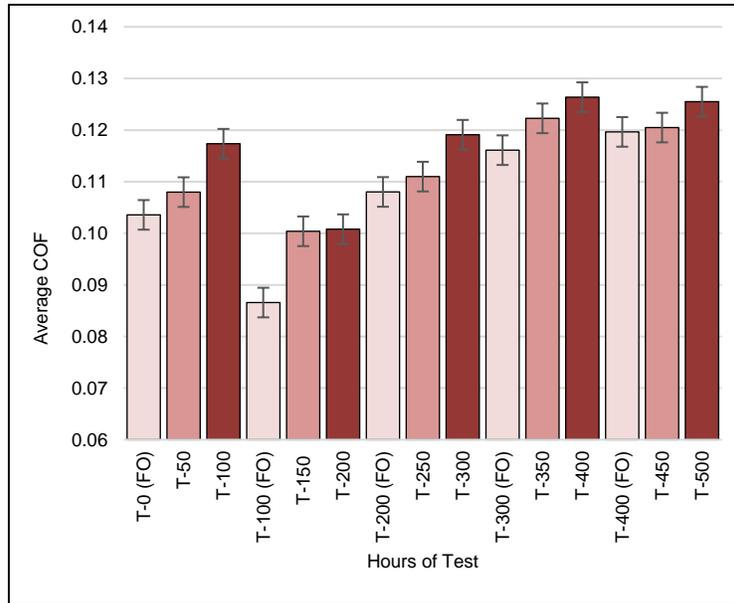
Figure 6: COF and average COF of diluted engine oil during the 500-hour endurance test.
