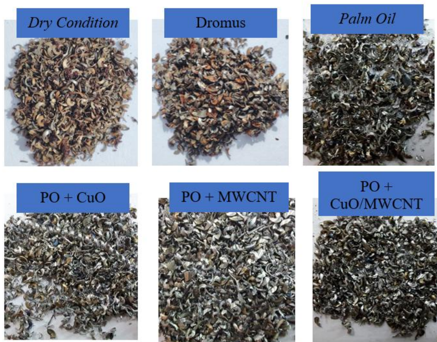
Figure 17: Chip color after application of cutting fluid Samples in CNC milling.
