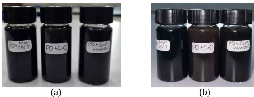
Figure 10: Sedimentation of cutting fluid samples at (a) 0 days and (b) 20 Days.
