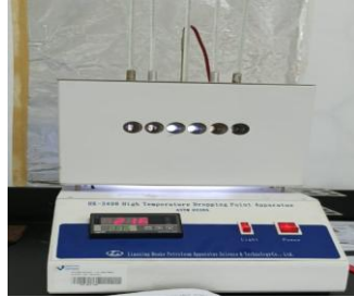
Figure 5: HK-3498 high temperature dropping point equipment (ASTM D2265).
