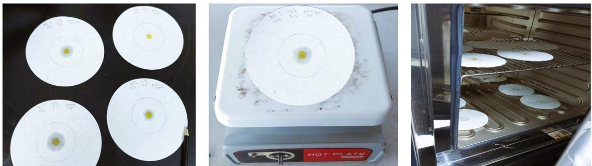
a) Oil bleeding of greases at room temperature after being left for ten days at room or ambient temperature
