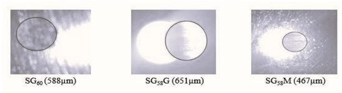
Figure 14: WSD images for each grease presence after the COF analysis.
