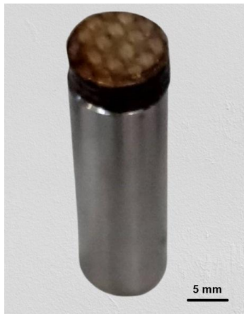
Figure 4: Wear test sample prepared as per ASTM G99 standard.
