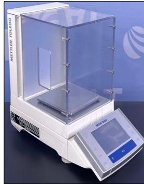
Figure 4: digital electronic weighing machine with a 10 4 gram precision.
