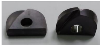
Figure 1: The cutting tool used in this study resembles the SFRT20 specification.
