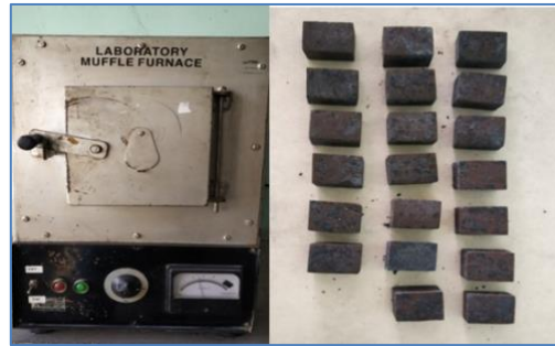
Figure 2: Muffle furnace and samples after Annealing.
