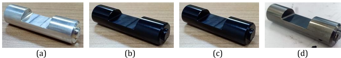
Figure 1: (a) Aluminum carrier, (b) Aluminum coated with Black anodized carrier, (c) Aluminum coated with Black anodized + Teflon carrier, and (d) Aluminum coated with Tetrahedral amorphous carbon (Ta-C:Ti) carrier.
