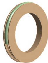
Figure 10: Three-dimensional model assembly drawing of traction wheel and wire rope.
