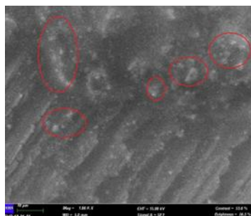
Figure 3: SEM micrograph captured at 1,000× magnification, revealing clusters of \text{TiO}_2 particles within the stir zone of Run 7.
